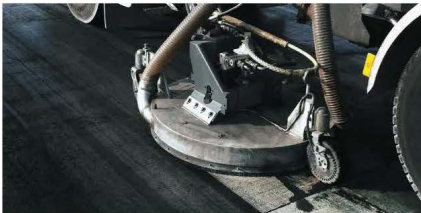
The surface cleaner in working position
