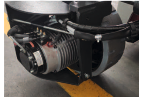
Motor electric AC; virare electrica pana la 90°
