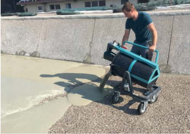
Optional accessory: pneumatic tires for uneven surfaces or for crossing underfloor heating.
