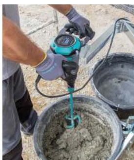
The mixer can be moved in all directions. Every sector in the bucket is reached.
