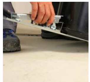
The adjustable foot treadle allows clamping of a wide range of bucket diameters
