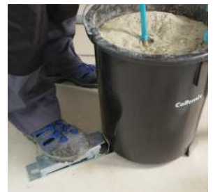
System with hand and foot: secure fixing with no forced postures
